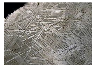
Picture 3 shows a close-up of Widmanstätten pattern etching.
